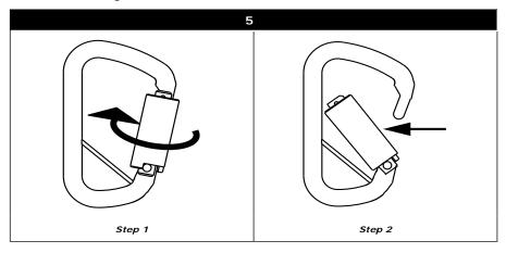
**B. CONNECT TRIPLE ACTION CARABINER**: Connect the carabiner to the connection point, rotate the gate clockwise, then pull gate up and push to the center of the carabiner. Position around a connection point, then release gate to close and lock. See Figure 6.
