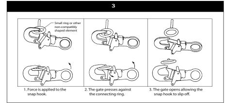
2.4 MAKING CONNECTIONS: Only self-locking snap hooks and/or carabiners shall be used with this equipment. Ensure all connectors are fully closed and locked and compatible. See Figure 4 Inappropriate Connections.
